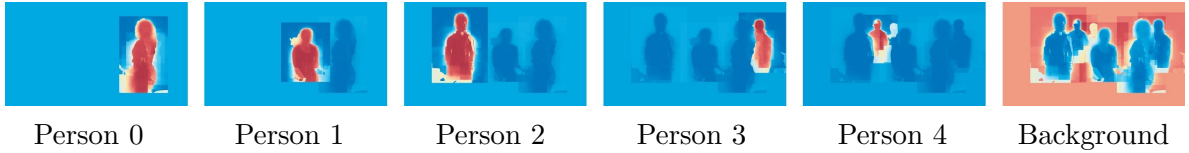
Figure 2.3 – Illustration of the occlusion-based unary costs for the example in Figure 2.1. From left to right we show the unary costs for persons labelled 0 – 4 and the background. The cost for a pixel to take a label (person or background) is denoted by the red (low) - blue (high) spectrum of colours. Here we observe the effect of accumulating the label likelihoods in a front-to-back order. For example, in the illustration for Person 4, a low cost (red) for taking label 4 is observed only for the pixels that are not occluded by the other people in front. ( Best viewed in colour. )
