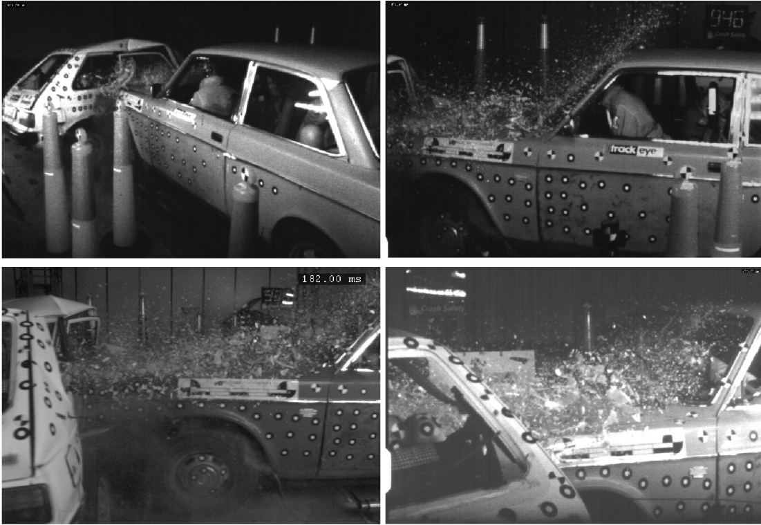
Figure 3.1: Images from four cameras in the Image Systems “cars” crash test sequence.
