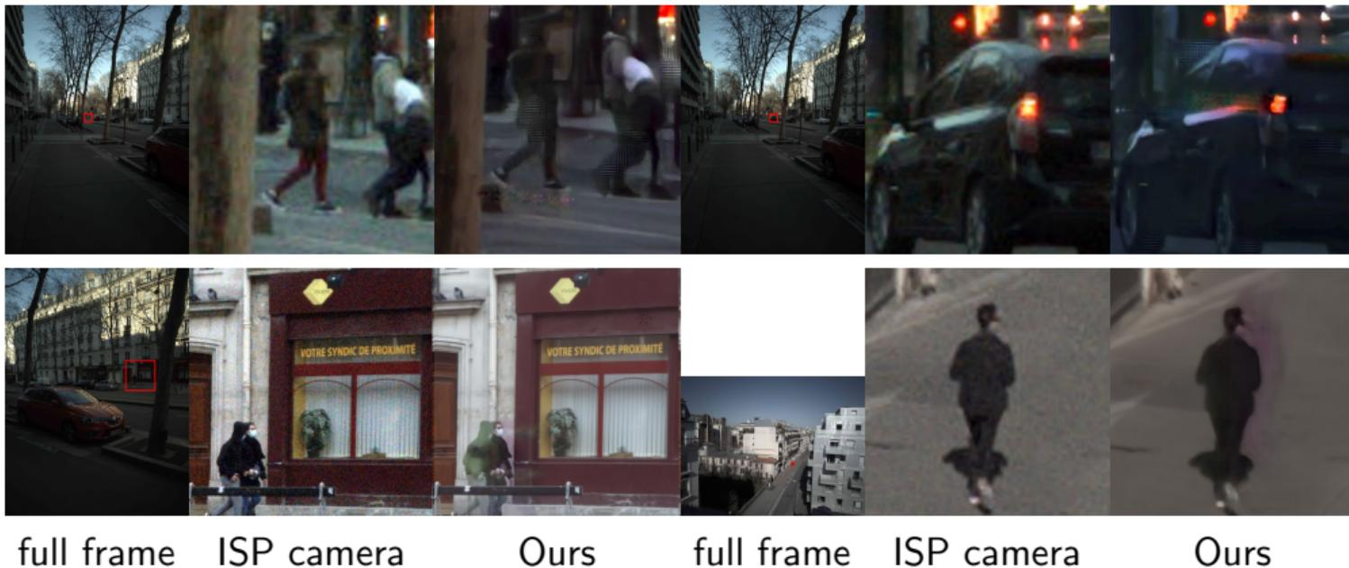
**Figure:** Misalignments artefacts due to moving objects in the scene. Our current implementation does not handle fast moving objects and then generates visual artefacts.
