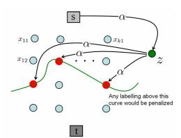
Figure 3. The graph construction for characterizing a general  $k^{th}$  order multi-label energy function. The variable z is an auxiliary node that is connected to k boolean nodes and the source with the same edge cost  $\alpha$ . As a result if all the k boolean nodes take the label 0 then the cost of the cut is 0. In all other cases there is a uniform cost of  $\alpha$ . This can be seen as a generalization of the graph construction given in [13].
