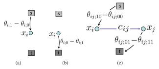
Figure 1. Converting an energy minimization problem to an stmincut problem [13]. (a) and (b) show unary potentials are represented using edges in the graph, while (c) shows the same for submodular pairwise potentials.
