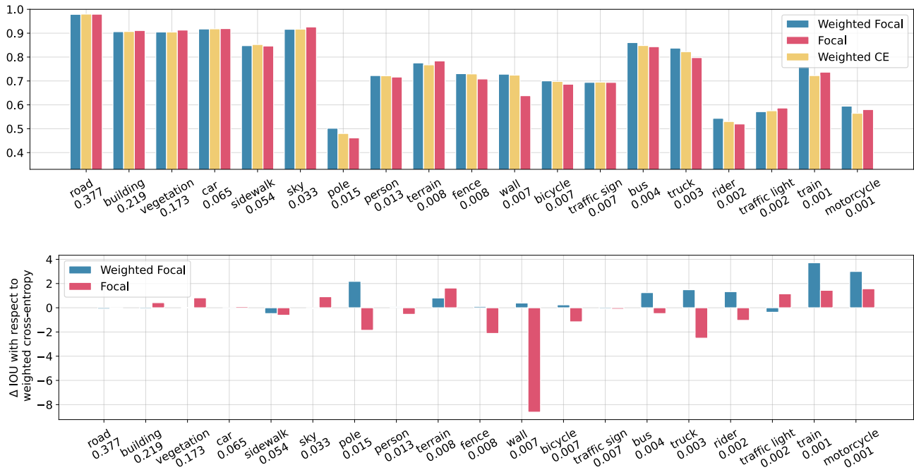
Figure S6. Top: Per-class IOU MF on Cityscapes with models trained with different loss functions using ConvNext-L backbone. Labels are sorted according to their frequency in the validation images, which is written below the class name. Bottom: Per-class difference in IOU MF of models trained with weighted and non-weighted focal loss w.r.t. the model trained with weighted cross-entropy (CE) loss.
