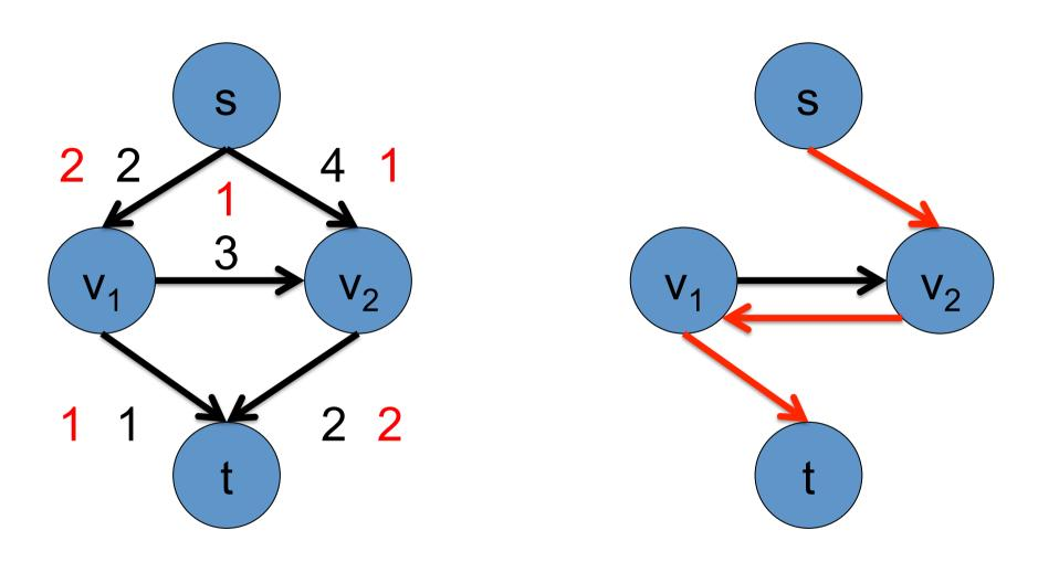
Choose maximum allowable value of K. Add K to  $(s,v_2)$  and  $(v_1,t)$ . Subtract K from  $(v_1,v_2)$ .
