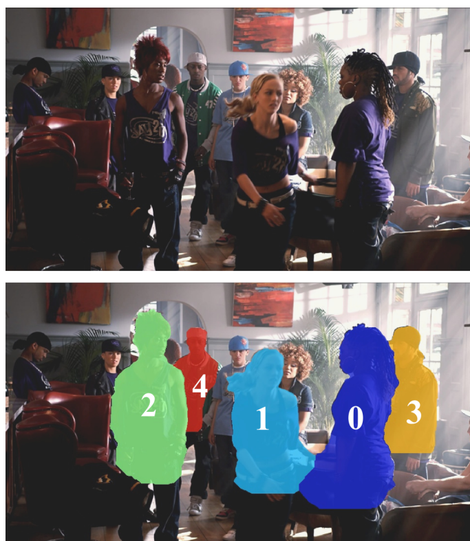
Figure 13. We segment multiple people in the scene, estimate their poses and relative front-to-back order, denoted by the numbers in the image below, in every frame of a video sequence.
