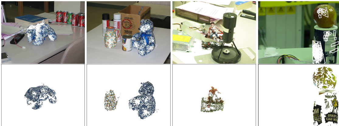
Figure 5: Object recognition experiments. The top row shows the model patches that were matched to the images, and the bottom row shows the models recognized, rendered in their estimated poses. Note that the teddy bear in the leftmost column is in a pose radically different from those used to acquire its model, and that there is a significant amount of clutter and occlusion in each image.
