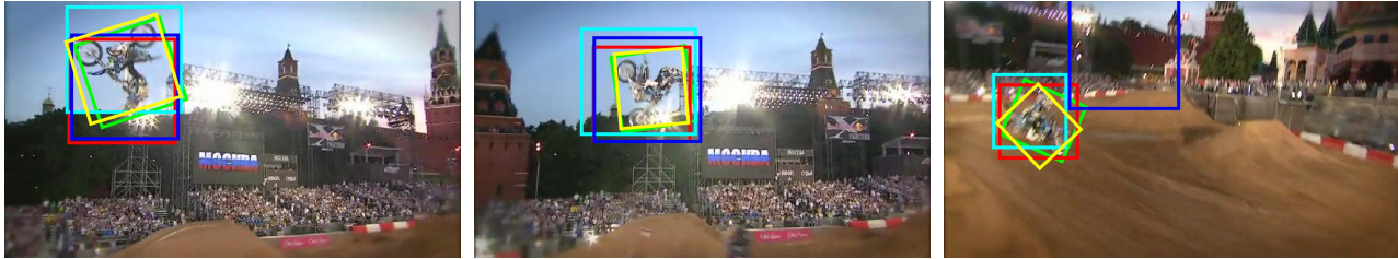
Figure 5. Sample result on the motocross sequence. We compare with several state-of-the-art trackers. Ground truth: green, Our result: yellow, DSST [12]: red, PLT 14 : cyan, Struck [19]: blue. Best viewed in pdf.
