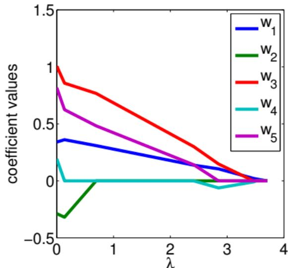
Figure: The regularization path of the Lasso is piecewise linear.
