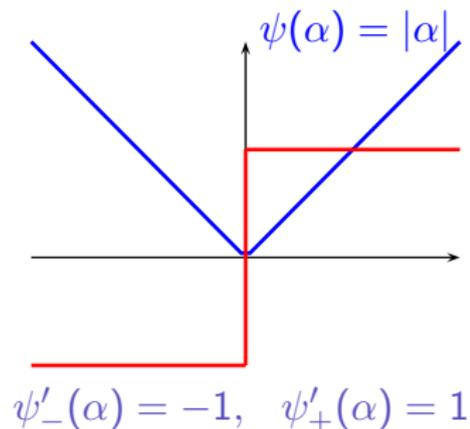
The gradient of the  $\ell_2$ -penalty vanishes when  $\alpha$  get close to 0. On its differentiable part, the norm of the gradient of the  $\ell_1$ -norm is constant.
