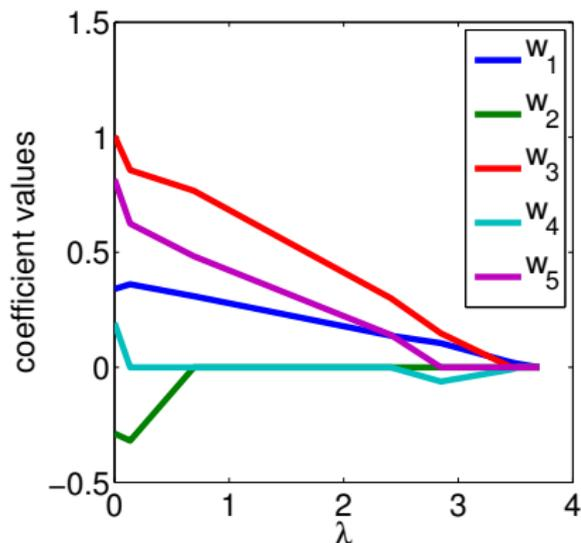
Figure: The regularization path of the Lasso.
