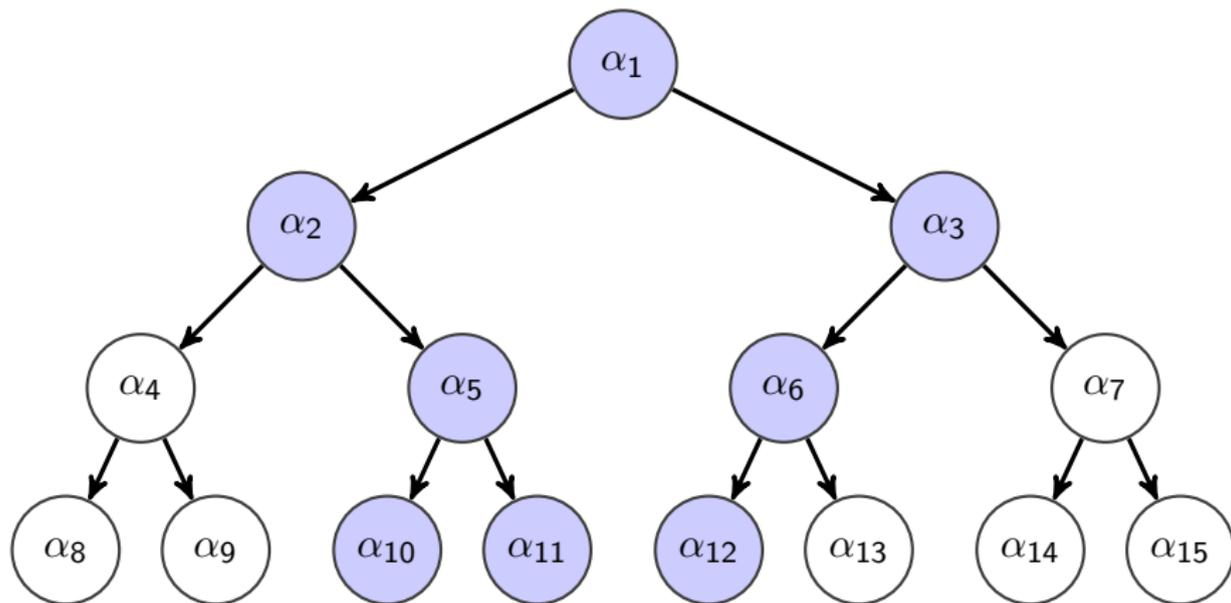
**Figure:** Illustration of a wavelet tree with four scales for one-dimensional signals. We also illustrate the zero-tree coding scheme [Shapiro, 1993].
